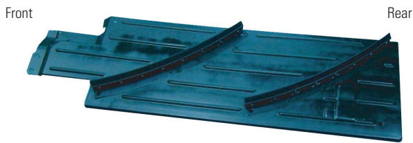
Fig. 8 Under floor air guide
